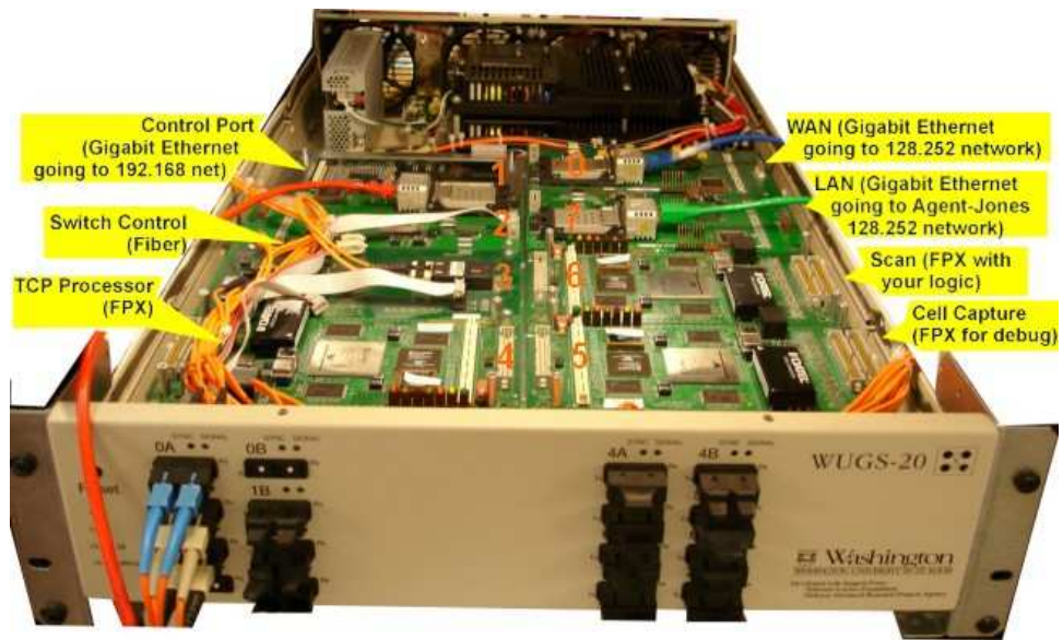
Figure 4.1: Photograph of the Network Processing Platform: A WUGS-20, three FPX platform boards, and three Gigabit Ethernet network interfaces
