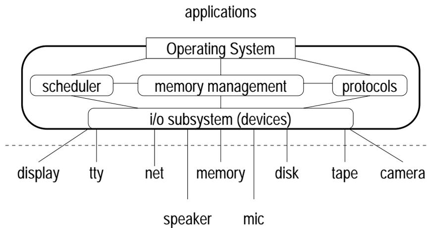
Figure 2: Types of I/O devices
