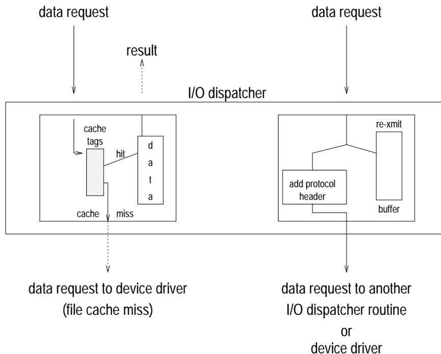
Figure 17: Two example paths through the I/O Dispatcher
