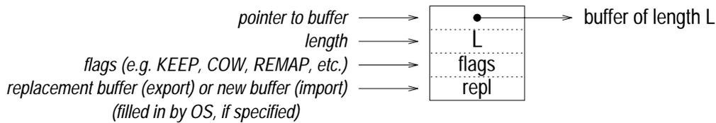
Figure 8: An example buffer vector structure
