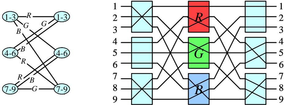
Figure 4. Simultaneous connection routing in  $C(n,n,r)$  using graph edge coloring
