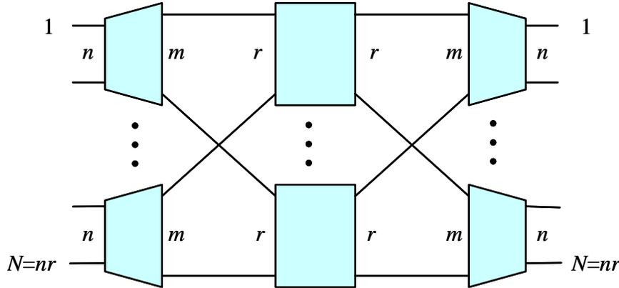
Figure 1. Symmetric three stage Clos network,  $C(n,m,r)$
