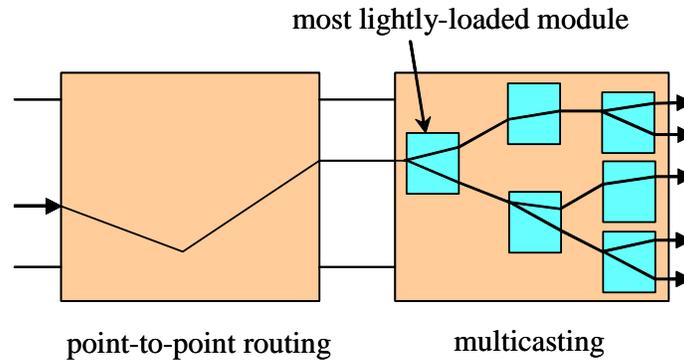
Figure 6 Adding multicast connection to cascaded Clos networks
