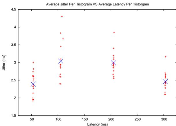
**Figure 4. Typical Jitter VS Latency per histogram plot as perceived by the Quake 3 server for clients**
