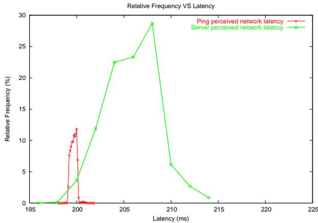
**Figure 3. Typical Relative Frequency VS Latency as perceived by ping and the Quake 3 server for clients**
