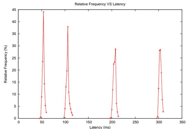
Figure 2. Typical Relative Frequency VS Latency as perceived by the Quake 3 server for clients
