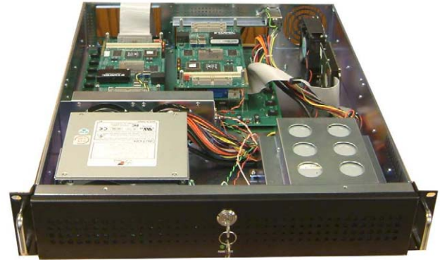
Figure 4: Rackmount case holds DED with FPX cards
