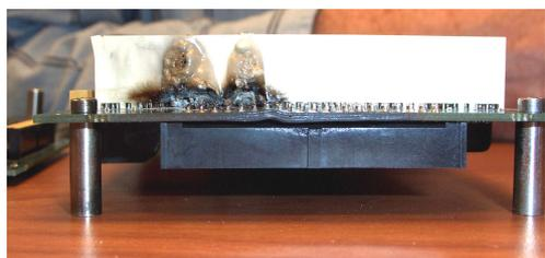
**Fig. 2.** Side view: Note how layers of the board were warped because of heat
