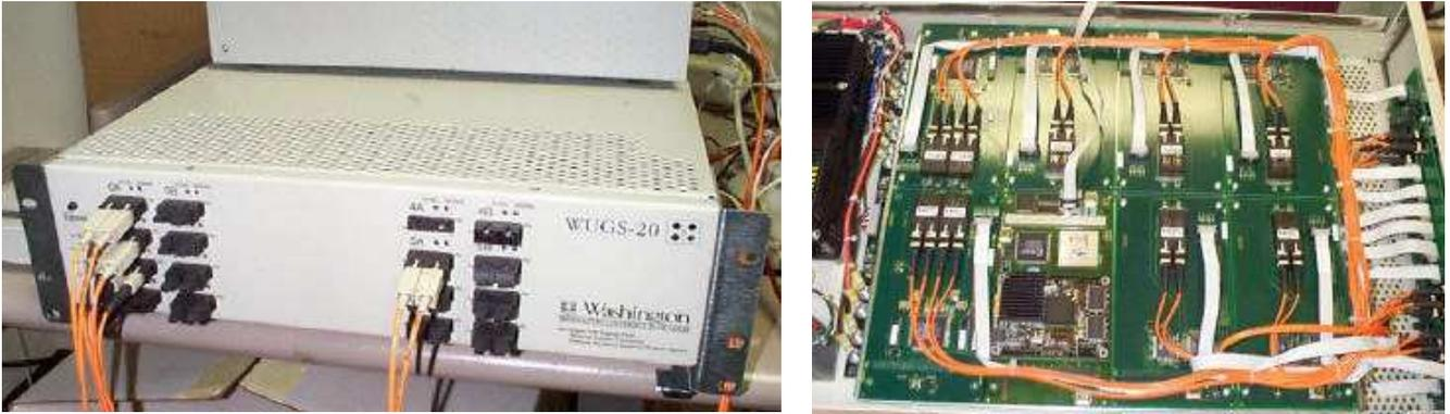
**Figure 2. Washington University Dynamically Extensible Router**
