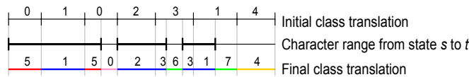
Figure 5: Example of the alphabet reduction algorithm when processing transitions leading from state s to t .
